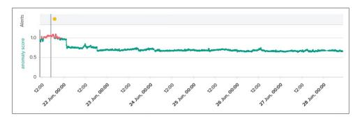
**Solution/Analysis:** The delivered Al/ML model for the air compression system successfully identified a process anomaly, pinpointing a drop in steam inlet temperature as the root cause. The model promptly alerted the user, enabling swift corrective action.
