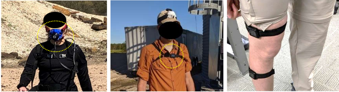
Figure 2. Instrumentation (left: K5 metabolic system, middle: chest IMU, right: lower limb IMUs).
