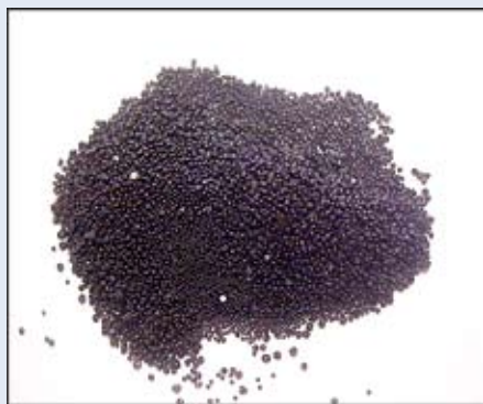
FIG. 6 Solid asphaltene pellets are easier to transport and store.
